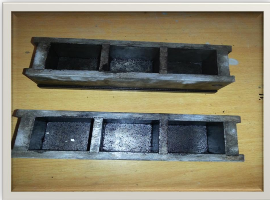
Figure II.4:Les moules cubiques 05*05*05 cm 3 .
